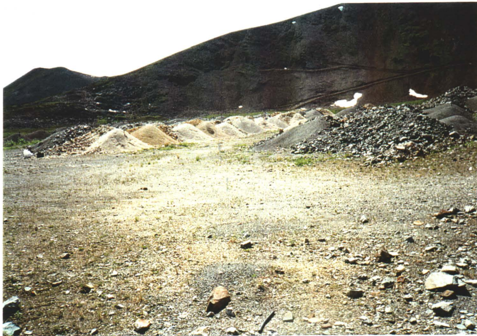
Photo 8. Ore piles (2 m X 4 m) extending westward containing 50% crushed rock (sorted to 1 cm diameter) and 50% muck sorted by round.
