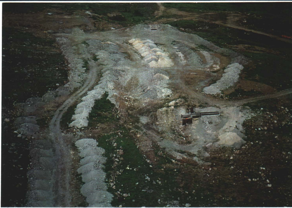
Photo 2. Aerial view of upper exploration area looking east. Note ore sample handling area (foreground), adit area (upper left) and access road to camp area at right.
