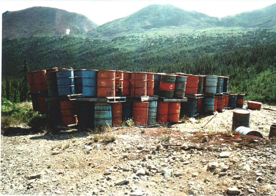
Photo 14. Detail of ore barrel storage area (total of 258 barrels on wood skids). Most barrels in this area were in good condition and contained graded ore sample material.
