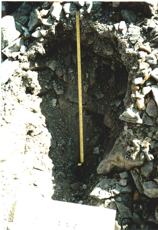
Photo 9. Detail of test pit LT-WR-R4 taken from muck portion of crushed reject ore pile material stockpiled on site.
