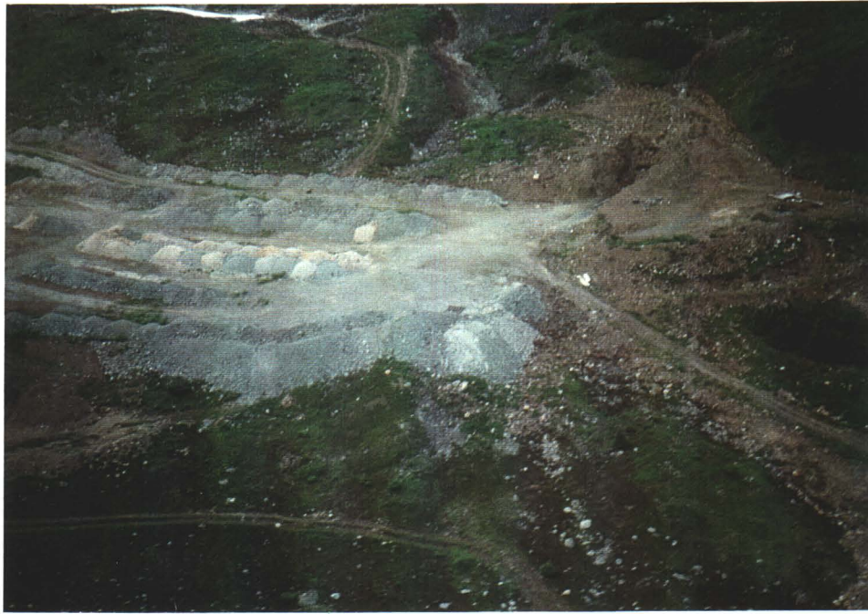
Photo 1. Aerial view of upper exploration area looking west. Note multitude of ore piles at left and adit entrance at upper right.
