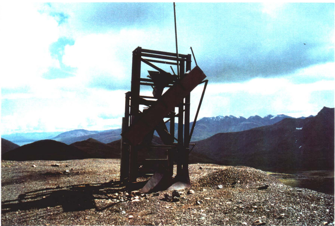
Photo 8. Ore sample splitter, viewed toward east.
