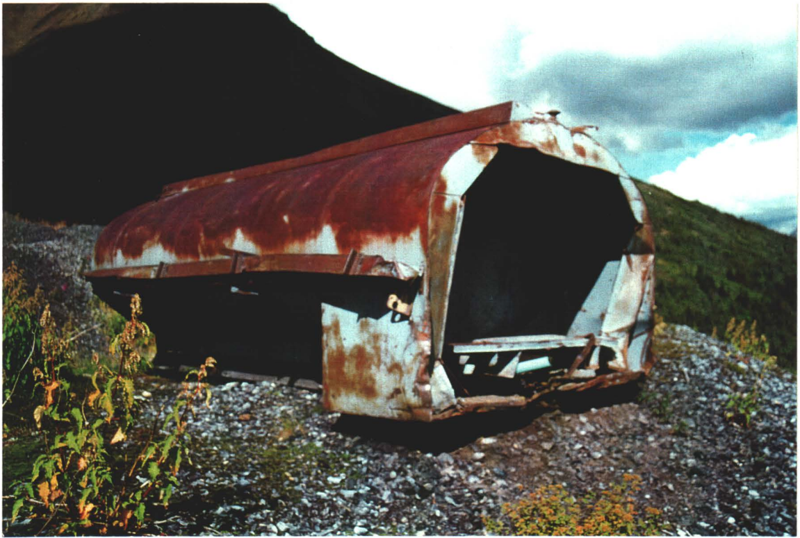
Photo 7. Bowser-style truck tank on mine access road at base of slope.
