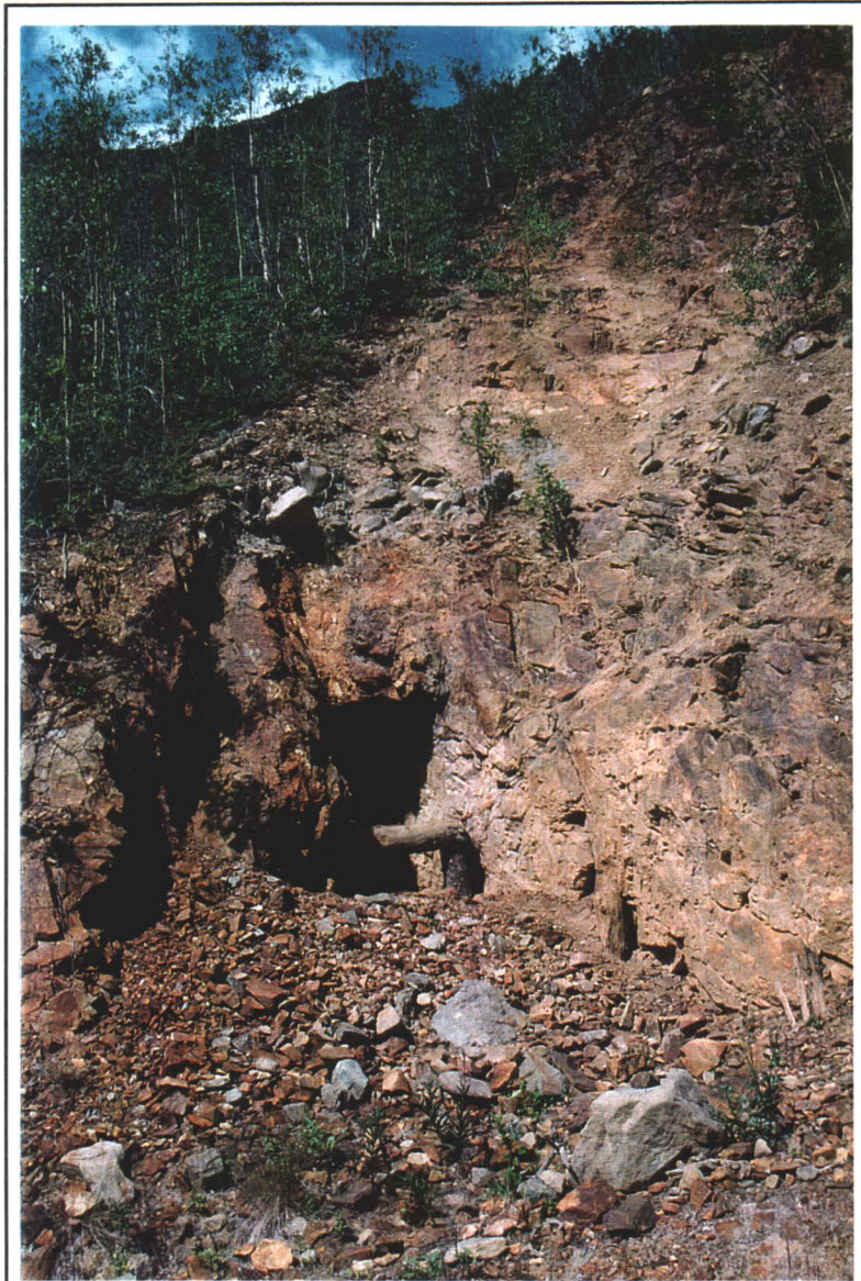
Photo # 6 - Middle Adits - Middle Site, Adit and Waste Rock
