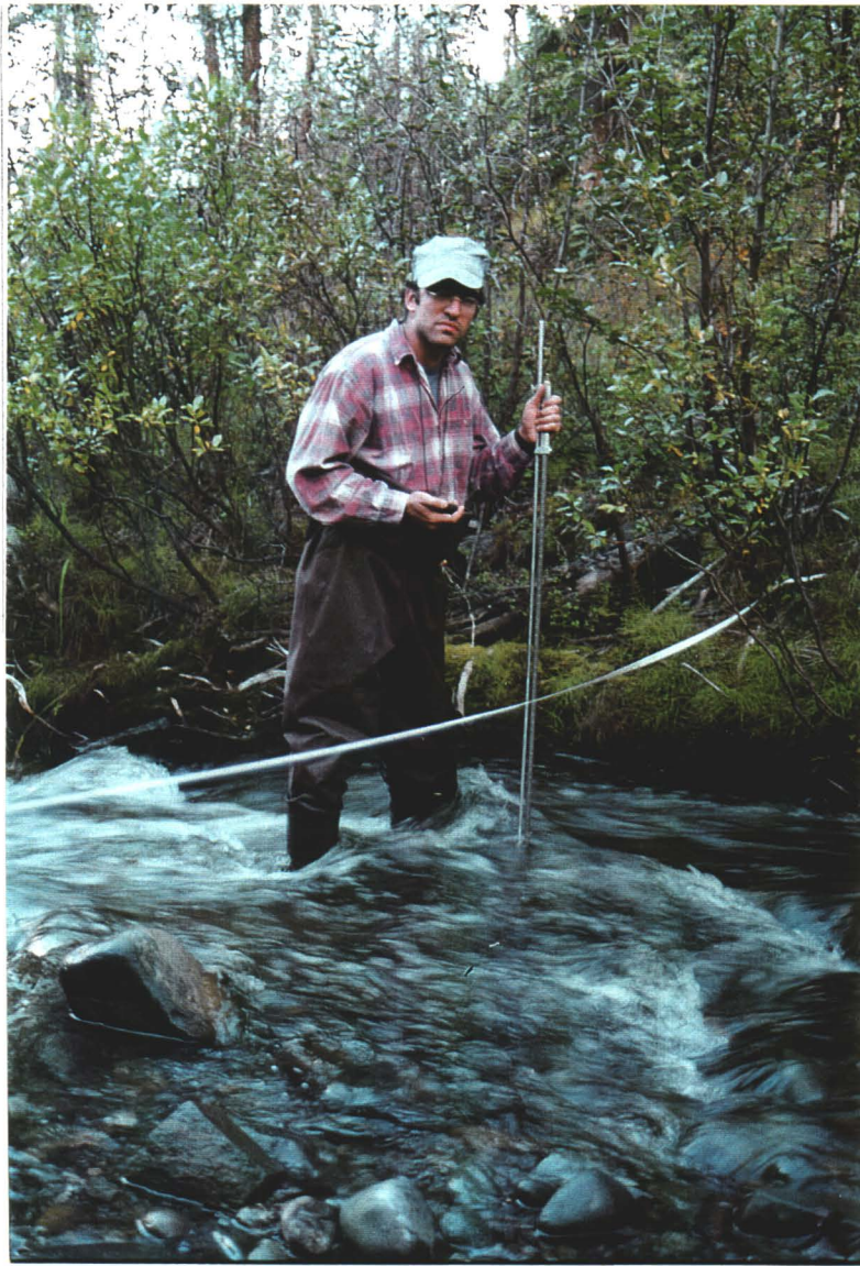
Photo 10. Christal Creek discharge measurement below toe of lower/eastern waste rock slope, 19 August 1997.
