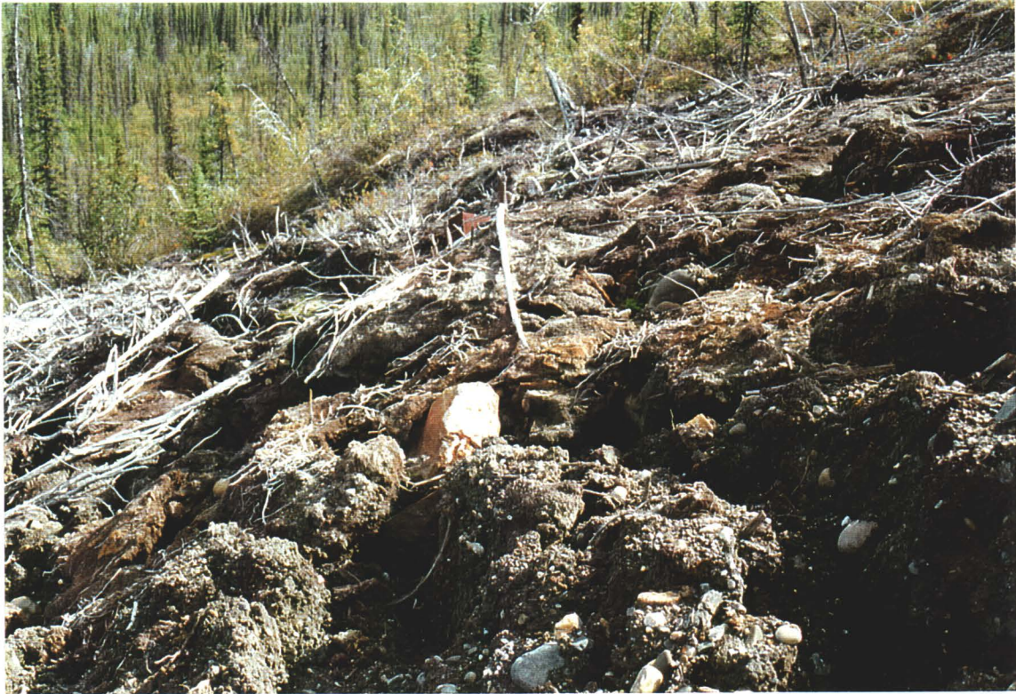
Photo 4. Slumped, eroded peaty overburden; note vegetation mortality caused by the disturbance of root systems.
