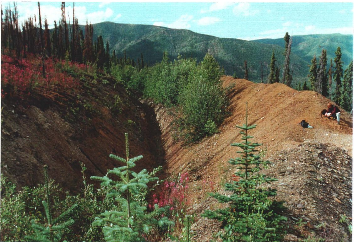
MN 6. "Trench 1" showing stained rock and overburden sidecast, and sample location OL/WR/Px1 .
