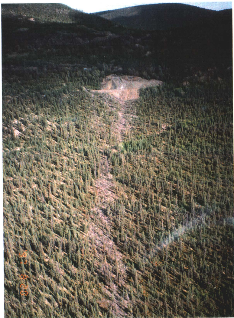
Photo #PE1: Looking east at waste rock pile near adit and stressed vegetation along slope. Note benched tailings.
