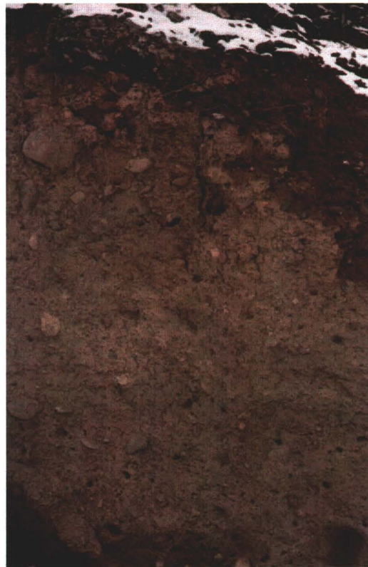
Photograph 15: Poorly sorted till material comprising the surficial sediments in a geotechnical test pit on the proposed heap leach site
