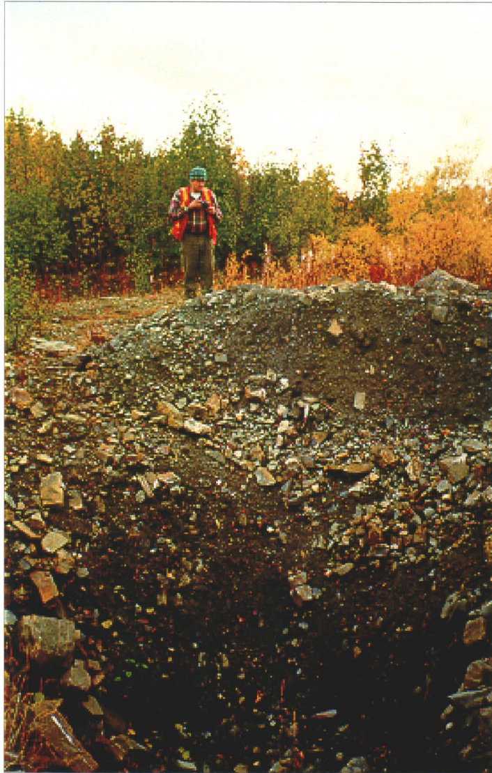
Photo 4-4: Photo of the collapsed western raise located directly above the main Dixie site. (Azimuth 210°)
