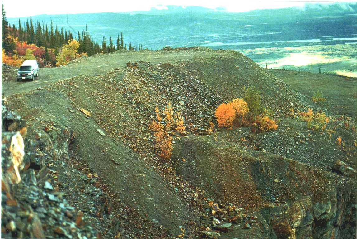
Photo 11-10. Waste rock dump located adjacent to the Sime #4 open pit (lower right-hand corner of photograph).
