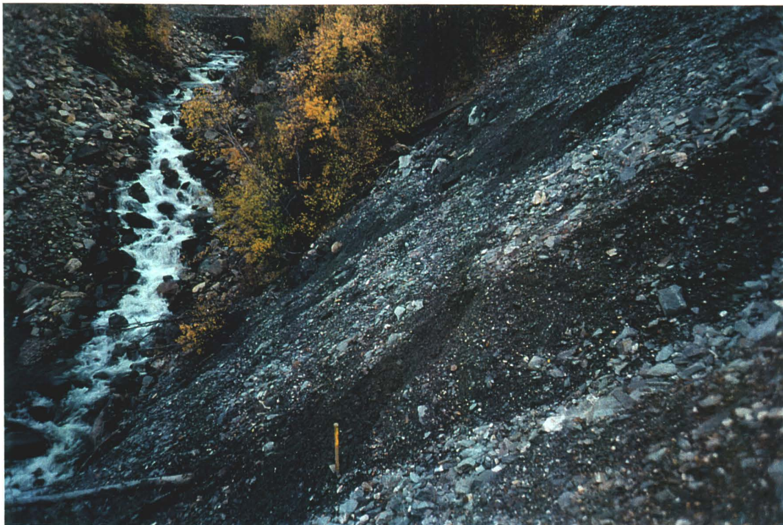
Photo 22-21 : Slumping evident in Bellekeno mine waste rock above Thunder Gulch creek. (Azimuth 160°)
