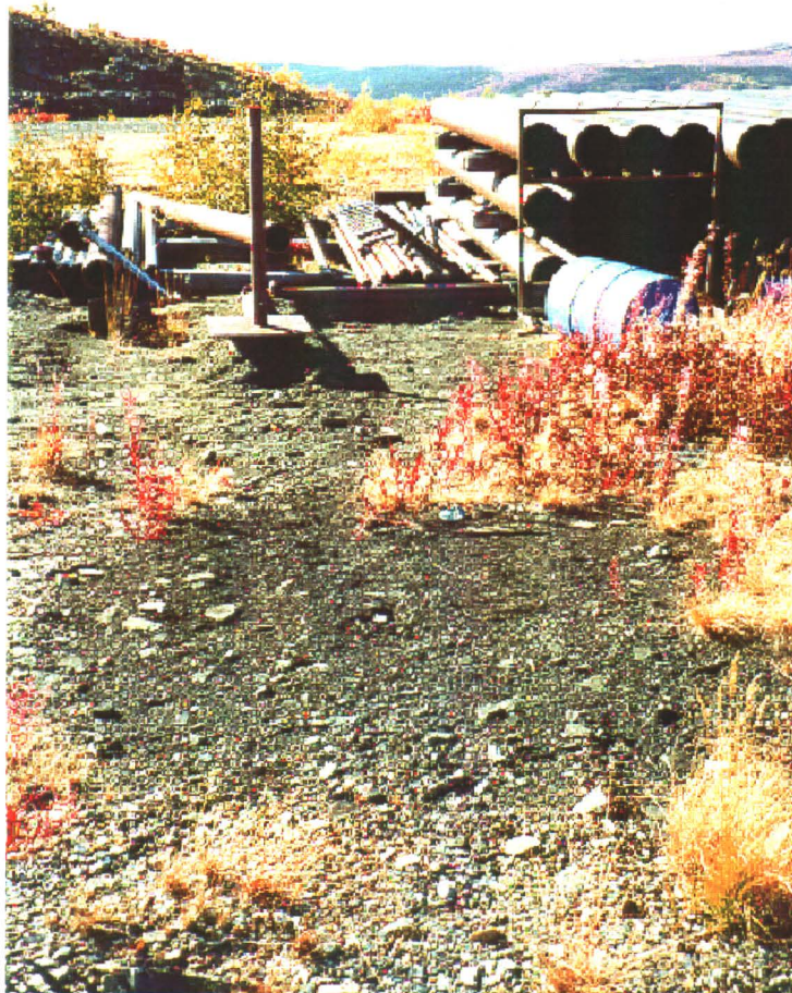
Photo 22-14: Drilling site with soil staining in foreground. Laydown of piping and empty hydraulic fluid barrel are in background.
