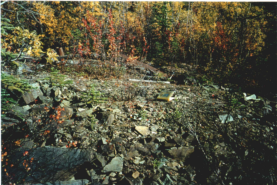
Photo 23-6: Rock dump from upper trench and adit (18m x 4m x 2m). Material comprised of approximately 80% colluvial soil and angular greenstone boulders.
