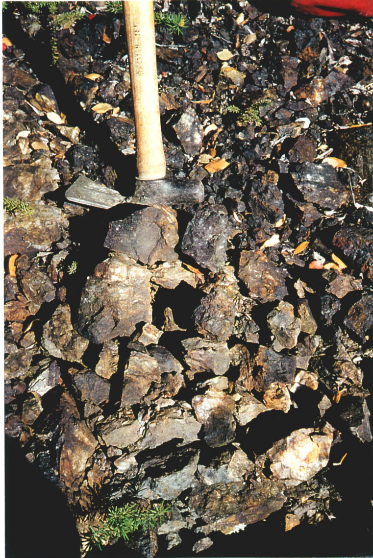
Photo 23-3: Close-up of strongly weathered, semi-massive galena-tetrahedrite siderite-quartz vein ore stockpile material (5m x 3m x 0.5m).
