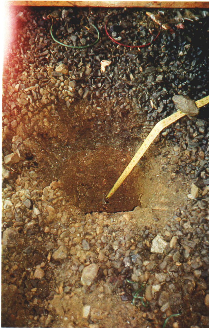
Photo 25-17: Test pit TP01 in Lucky Queen shop. Note heavy oil stain on surface gravel.
