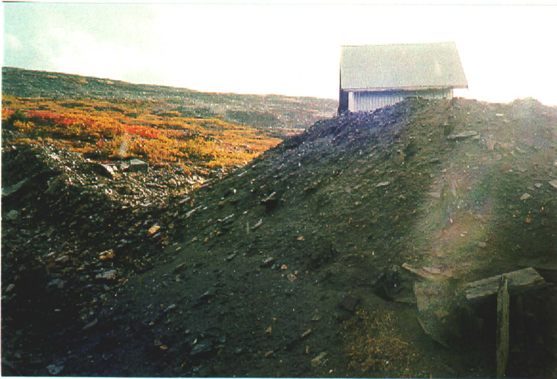
Photo 26-6: Trench east of shaft building. Note waste rock dump from underground development forming slope at right of photo. Photo Direction (Azimuth 130°)
