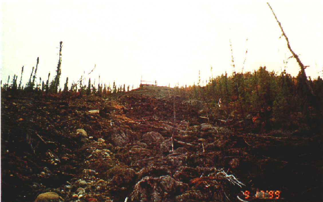
Photo 57-4: Waste rock below lower workings. Note extensive vegetation kill zone.
