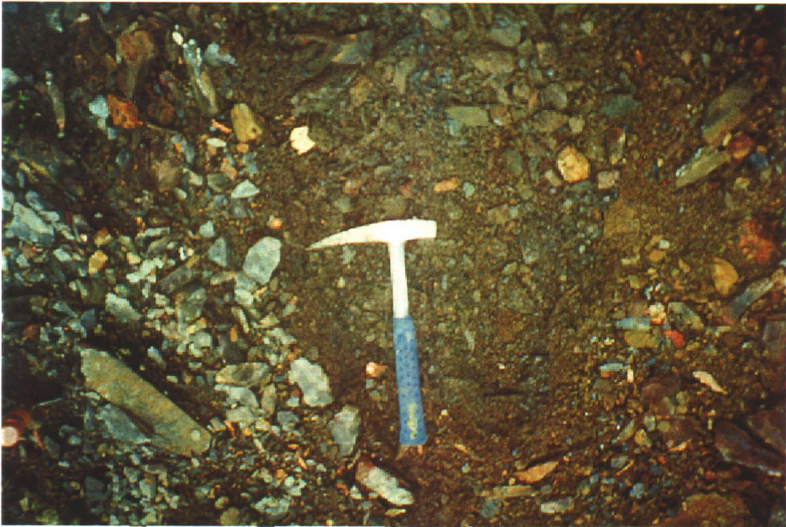
Photo 63-3: Test pit from waste rock pile #2. Note the shallow oxidation horizon. (Azimuth 170°)
