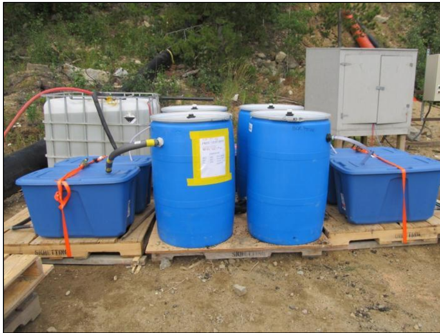
Figure 1. Pilot-scale bioreactors at Minto Mine (Picture taken in August 2014).
