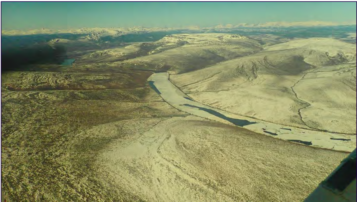
FIGURE 6.4.4. INTACT ICE COVER AT Km 188 AND JUXTAPOSED ICE JAM UPSTREAM OF THAT POINT ON MAY 12 AT 4:45 PM.
