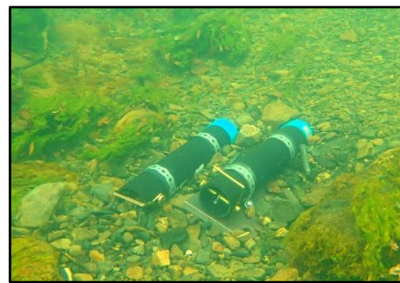
Figure 1. A pair of anchored plates at the bed of a stream to which the aquatic sensors are attached.
