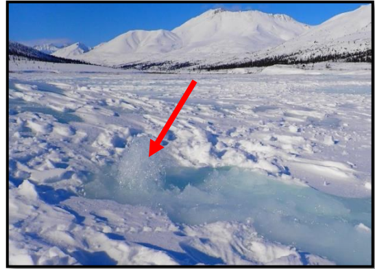
Figure 3. Pressure-driven overflow through an augered hole at km 72 on the Dempster highway on Apr 4, 2024.
