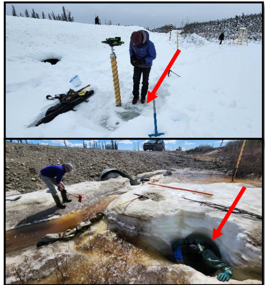
Figure 4. location of an augered hole at km 32.6 on the Dempster highway in March 2023 (top) and the expansion of this drainage hole by early May 2023 (bottom).
