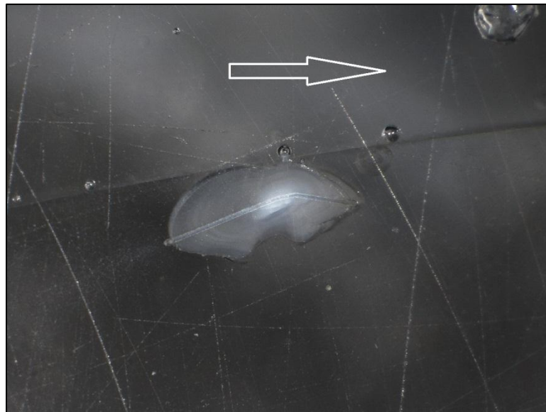
Figure 12 Slimy Sculpin otolith (sample CC7) after LA-ICP-MS analysis (arrow indicates the direction of the laser path across the sample)
