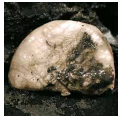
Figure 2.10: Gas hydrates in clay-rich sediments. Gas hydrates have been discovered in rich deposits characterized by dense arrays of nodules and hydrate-filled fractures in clay-rich sediments. Left: CT image of a core samples collected offshore India in 2006. The hydrate-filled veins appear as white (from a paper by Rees et al. 2011, published by JMPG, permission would be needed). Above pictures, gas hydrate samples (courtesy NGHP Expedition-01 science party).
