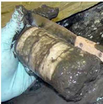
Figure 2.10: Gas hydrates in clay-rich sediments. Gas hydrates have been discovered in rich deposits characterized by dense arrays of nodules and hydrate-filled fractures in clay-rich sediments. Left: CT image of a core samples collected offshore India in 2006. The hydrate-filled veins appear as white (from a paper by Rees et al. 2011, published by JMPG, permission would be needed). Above pictures, gas hydrate samples (courtesy NGHP Expedition-01 science party).
