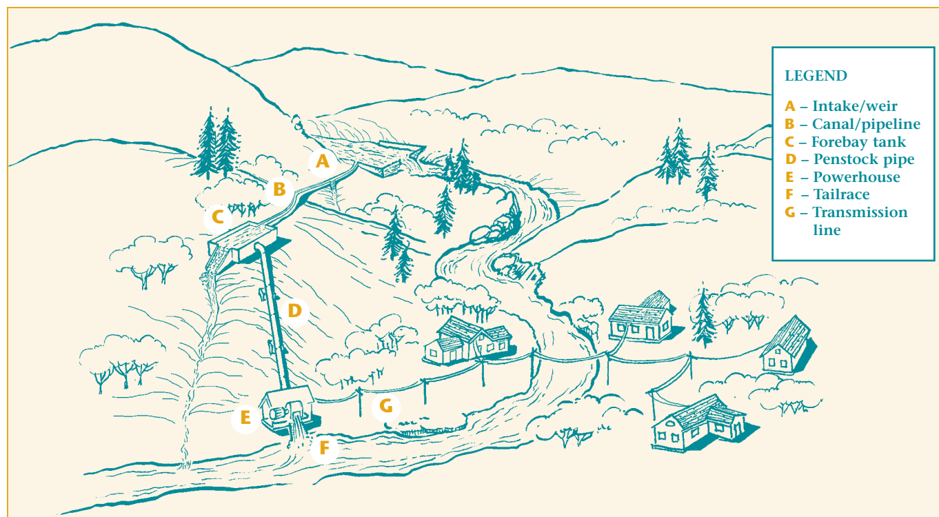
Figure 2. Principal components of a micro-hydropower system
