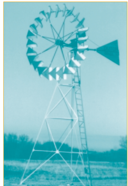
▲ Mechanical water pumping system.
