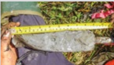
Core sample of mineral soil.
