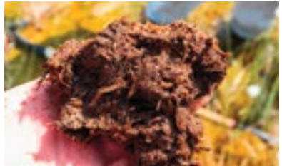
Organic soil (peat) with visible fibrous plant materials.
