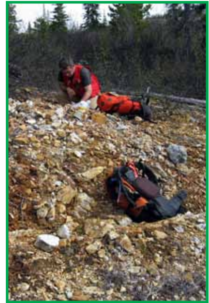
Road cuts, old trenches and exploration workings are often sampled as part of preliminary geologic evaluation of sites. When collecting samples off claims avoid using flagging or spray paint.
