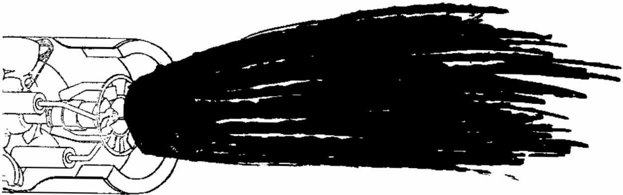
FIG. 1 CORRECT RETENTION - FLAME SHOULD BURN OFF THE 12 BLADE SPINNER APPROXIMATELY 1/4" TO 1/2".
