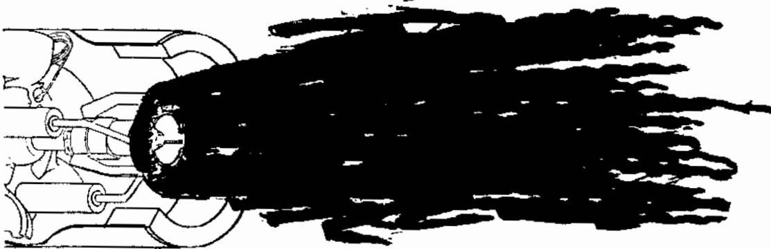
FIG. 2 FLAME IMPINGEMENT - TO CORRECT THIS PULL THE DRAWER ASSEMBLY BACK.
