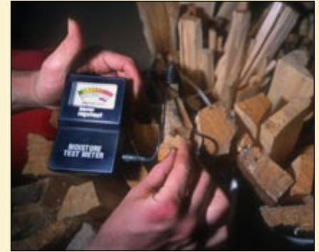
Wood moisture testers are available at hardware stores. Cathie Archbould
