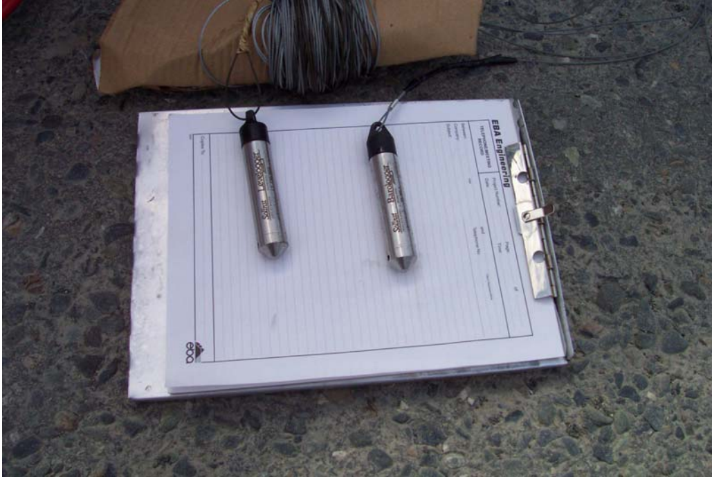
Photograph 8: Solinst Levelogger® and Barologger® dataloggers for monitoring water level and barometric fluctuations during pumping test.
