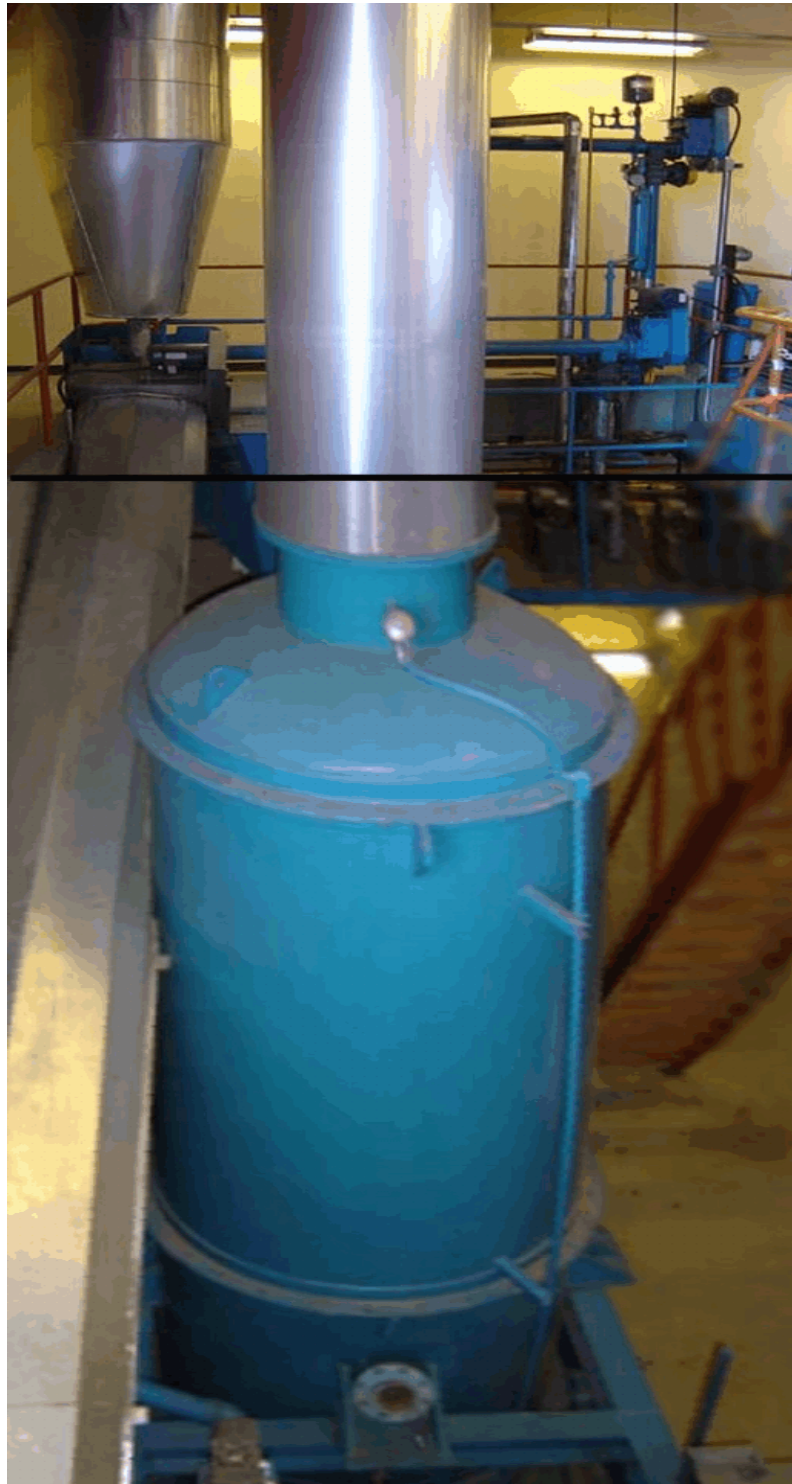
Figure 7. Refractory-lined gasifier vessel
