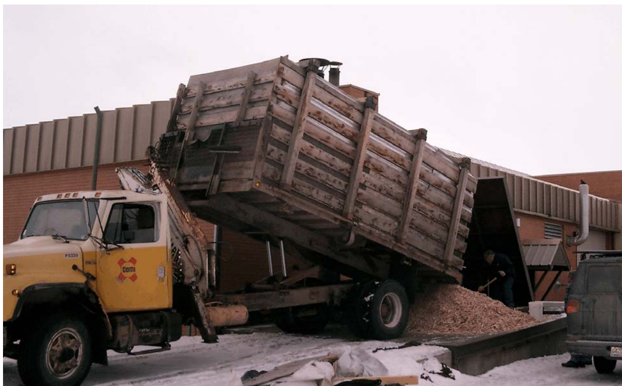
Figure 2. Truck dumping wood chips into underground bunker
