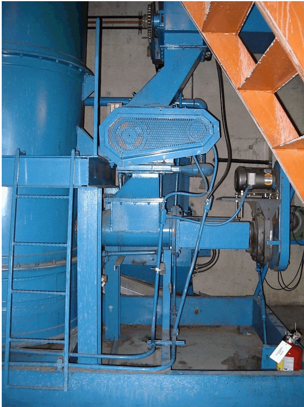
Figure 4. Wood chip feed system (airlock valve)
