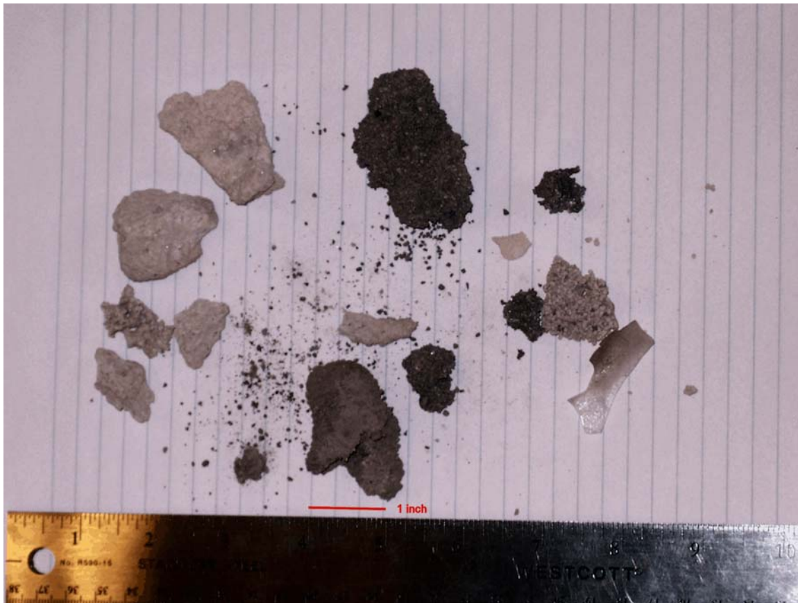
Figure 11. “Chunks” removed from gasifier during pre-test evaluation
