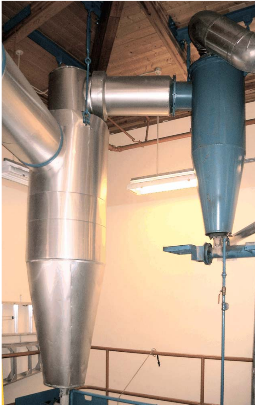
Figure 12. Cyclones to remove ash from “syngas” stream
