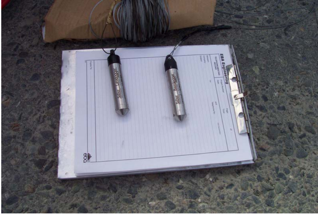
Photograph 8: Solinst Levellogger® and Barologger® dataloggers for monitoring water level and barometric fluctuations during pumping test.
