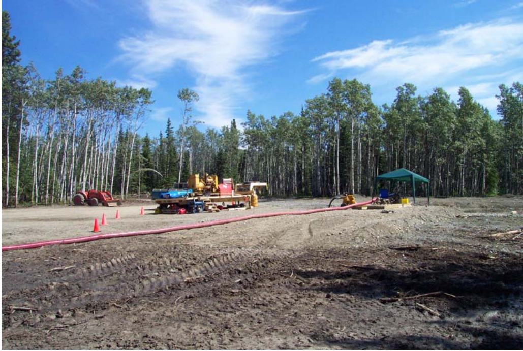
Photograph 2: Set-up for pumping test. Note: Generator on trailer deck (left), trash pump beside wellhead, canopy over well head (right) and discharge line running north-west from wellhead.
