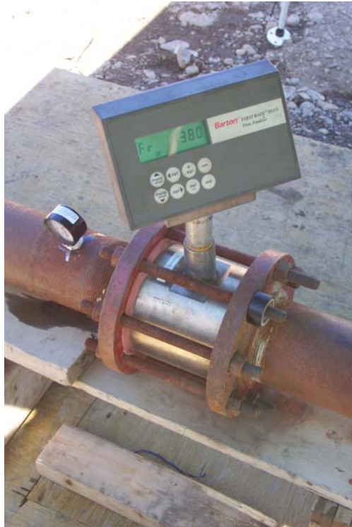
Photograph 6: Barton flow totalizer flow meter measuring instant and total flow during second step of pump test (380 Usgpm)
