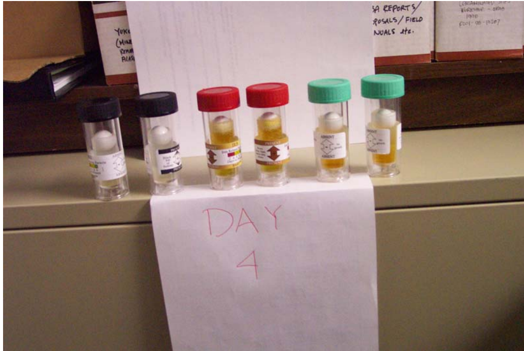
Photograph 10: Biological Reactivity Test (BART) on day 4. SRB (sulphate reducing) on left (black), IRB (iron reducing) in middle (red) and SLYM (slime forming) on right (green).
