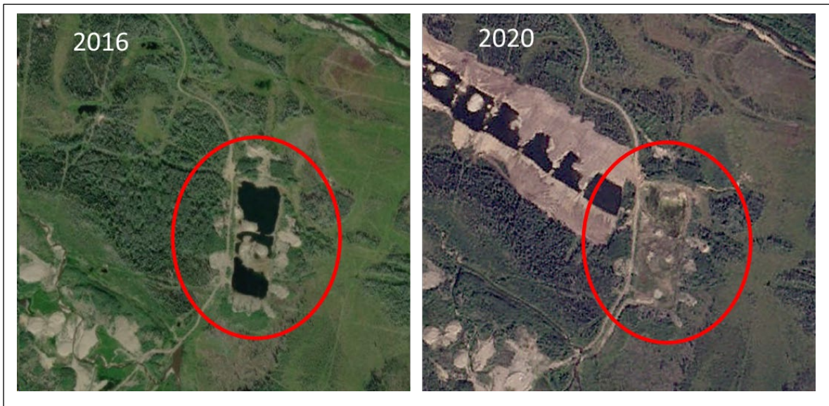
Figure 8. Satellite imagery of Site 1991 in 2016 and 2020, showing how the site was reworked with the addition of sediments from operations to the west prior to 2020.
