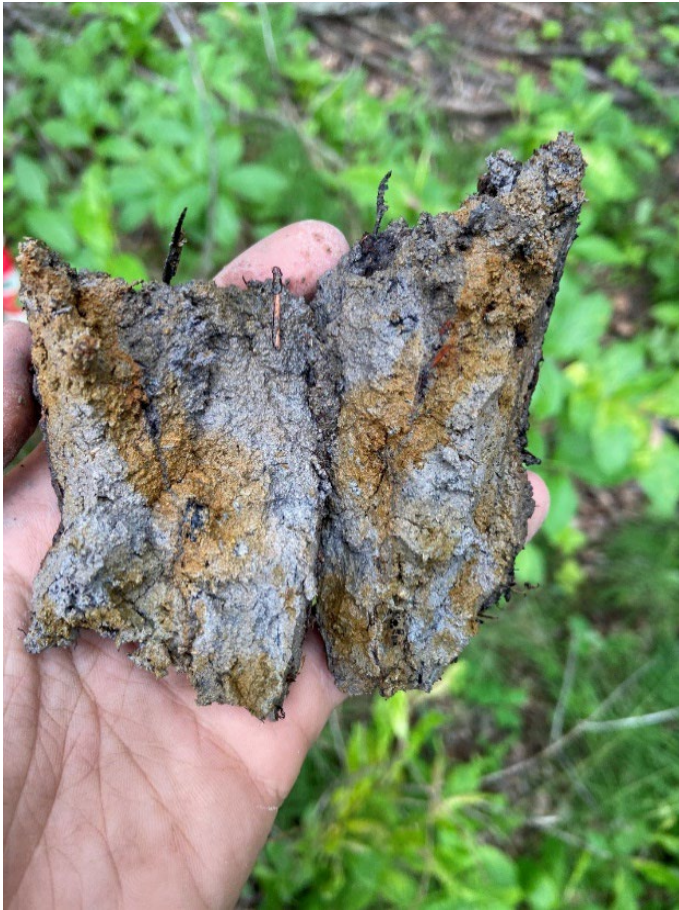
Figure A5-1A soil sample showing gleying (grey background) with prominent mottles (rusty red).
