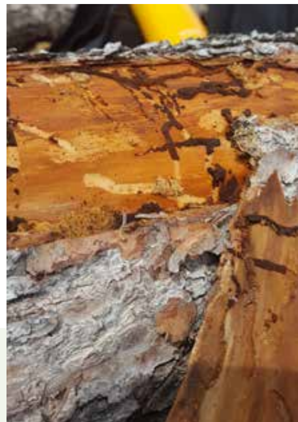
Photo 29 Wood borer larvae and tunnels on decked wood.
