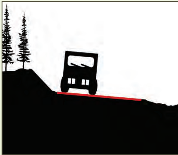
On roads with gentle grades, roads can be sloped so that the downsloped side is slightly lower than the upslope to allow drainage to the downsloped side.
