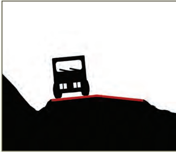
Roads should be crowned to shed water.
