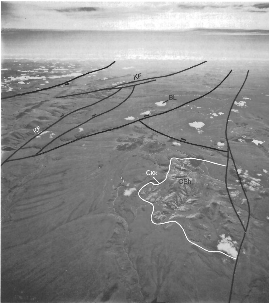
Figure 3.6. Rapid Fault Array in Rapid Depression at the headwaters of Blow River, Blow River and Davidson Mountains map area, Yukon Territory. Conglomerate and sandstone of Lower Carboniferous Kekiktuk Formation (CKK) lie unconformably upon slaty argillite (OSh), presumed to be coeval with the lower and middle Paleozoic Road River Formation. Downthrown walls are identified by black dashes. KF is Kaltag Fault; BL is Bonnet Lake. NAPL oblique photo T13R-114, looking south.
