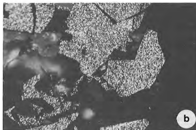
Figure 6. Heat affected bitumen showing fine grained mosaic texture and high anisotropy, Chads Creek B-64, 3390 m. Photographs taken in incident white light. Long axis 240 \mu\text{m} . a. Partially crossed polars and b. microscope stage is rotated 90° to show the anisotropy. Mf = fine grained mosaic.
