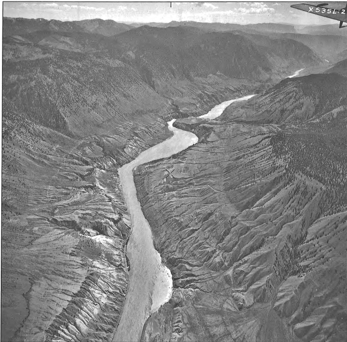
Figure 6. Dissected Quaternary fill in Fraser River valley north of Lillooet, British Columbia. Landslides from the steep bluffs bordering this and other rivers in western Canada have, on occasion, failed and impounded short-lived lakes. (Province of British Columbia airphoto BC1087-46).
