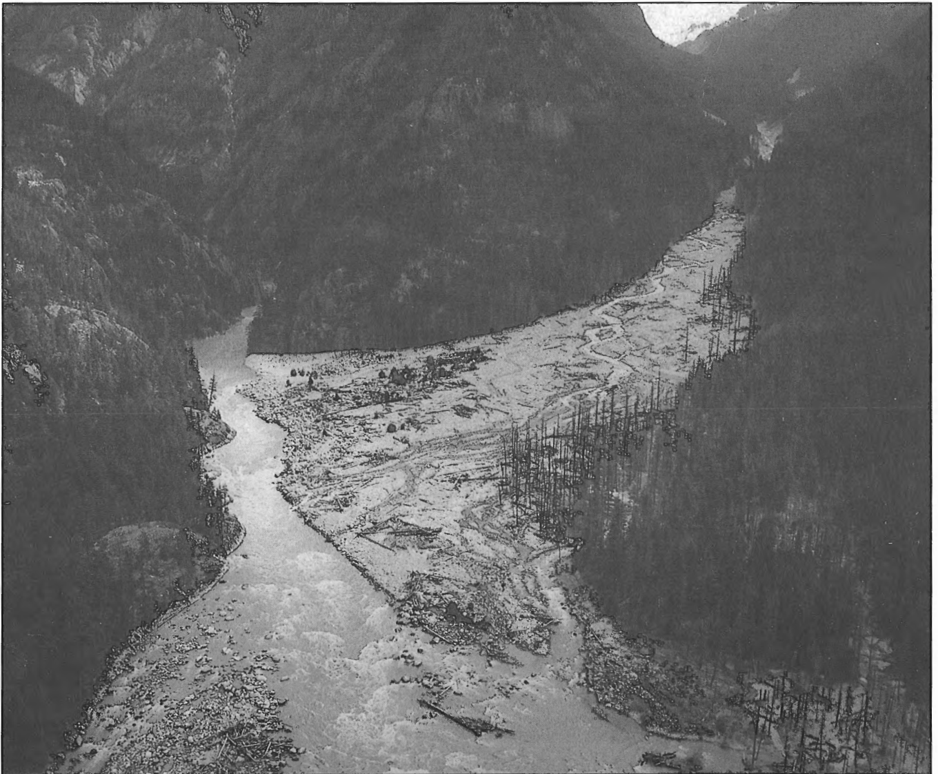
Figure 22. Fan at the mouth of Klattasine Creek. Bouldery debris deposited by the Klattasine Creek debris flow temporarily blocked Homathko River to form a lake. (Fig. 5 of Clague et al., 1985).
