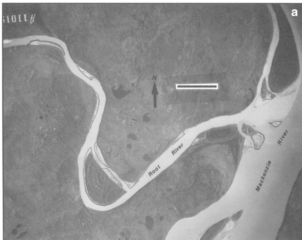
Figure B4. Sequence of aerial photographs of the Root River study reach a ) 1947 (NAPL A11019-12), b ) 1961 (NAPL A17496-17), and c ) 1977 (NAPL A24725-203); the black bar on each photograph represents one kilometre. The greater number of river bars in b ) reflects a lower river stage than in a ) and c ). Some of the bars in a ) have been outlined and shaded to enhance their profile.
