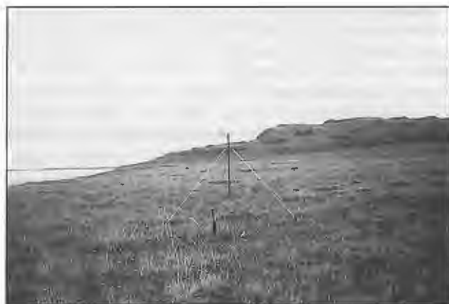
Figure 2. View of site 90 TT 9, Coral Bay, Mackenzie Delta, four years after jet-drilling the hole for the thaw tube with heave scribe (foreground). The ground temperature data logger is buried near the base of the air temperature screen.
