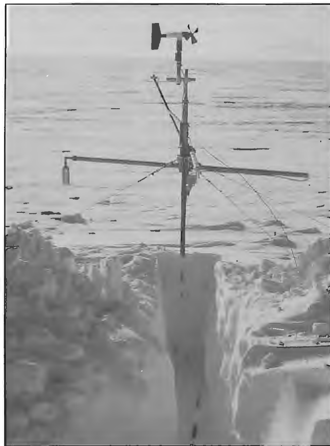
Figure 2. Agassiz Ice Cap 1977 borehole site autostation mast with two snow depth sensors (one hidden behind mast), Gill radiation shield, and wind sensor. The data logger enclosure is buried under the snow. The instrumentation has been provided and maintained in the past few years by Campbell Scientific Canada Corporation as part of a Industrial Partners Program, testing autostation technology in the severe climatic conditions experienced on high arctic ice caps. (photo: M. Waszkiewicz)
