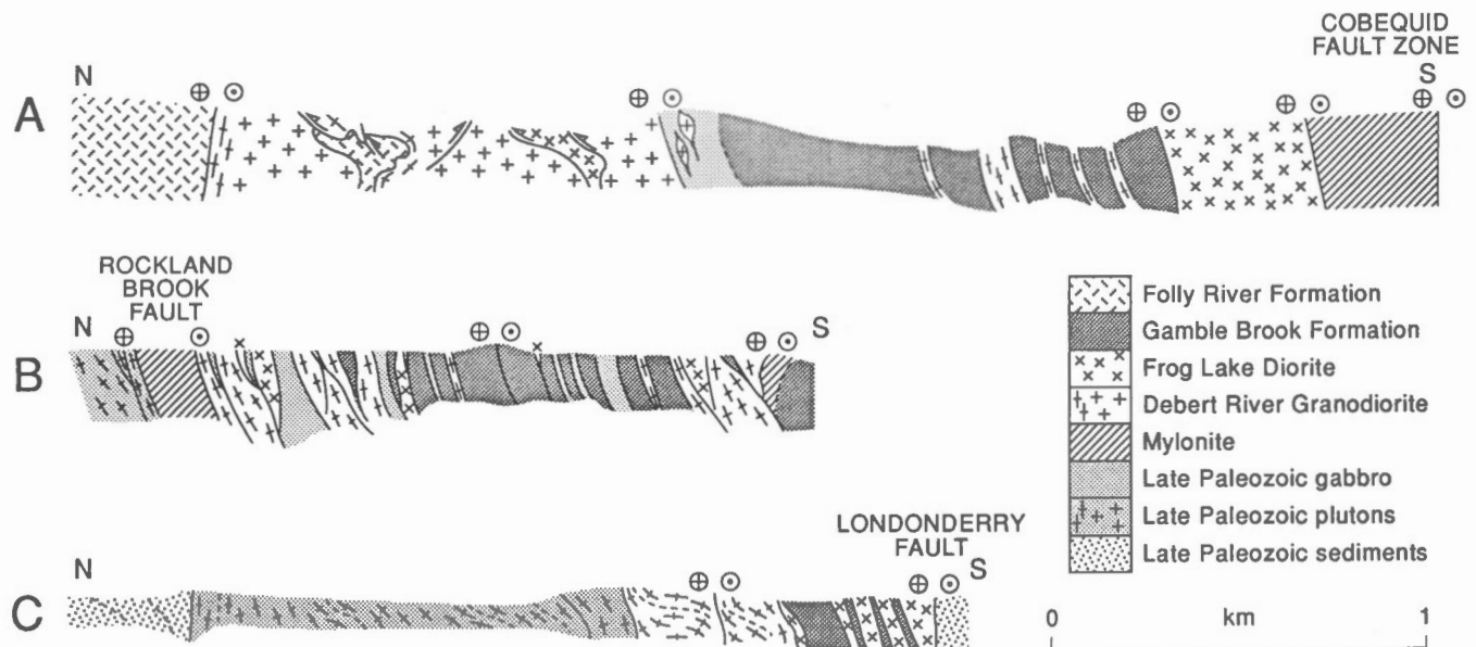
Figure 2. Schematic cross-section of the Neoproterozoic rocks south of the Rockland Brook fault. (A) along the Debert River (D in Fig. 1); (B) north of Londonderry on the Higgins Mountain road (GV in Fig. 1); (C) Portapique River (P in Fig. 1).
