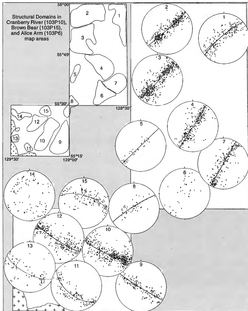
Figure 10. Map of structural domains with stereonets. Stereonets are lower hemisphere projections of poles to bedding, plotted on Schmidt nets.
