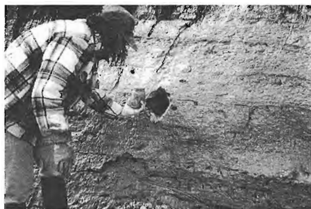
Figure 3. Close-up of bedded silty-clay deposit showing silty-clay layers separated by thin (dark) bands of clay-rich material. D.S. collecting sample for testing. Note the white, shelly material in lower right corner of the photo. GSC photo 1999-008D
