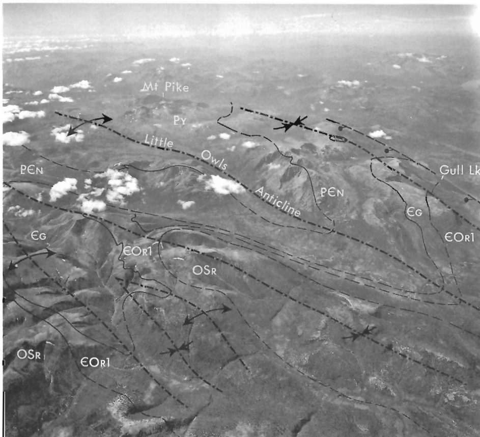
Figure 68. Oblique areal view southeasterly toward Mount Pike, showing distribution of strata, Little Owls Anticline, and other unnamed structures. Mountainous, yet recessive topography is typical of Selwyn Mountains, which are largely underlain by chert and clastic strata. Map units shown include the Yusezyu ( Py ), Narchilla ( PCN ), Gull Lake ( EG ), and Rabbitkettle ( EO1 ) formations and the Road River Group ( OSR ). Dots indicate downthrown side of fault that trends through Gull Lake (Canadian Government photo T11-75R). GSC 204923-C.
