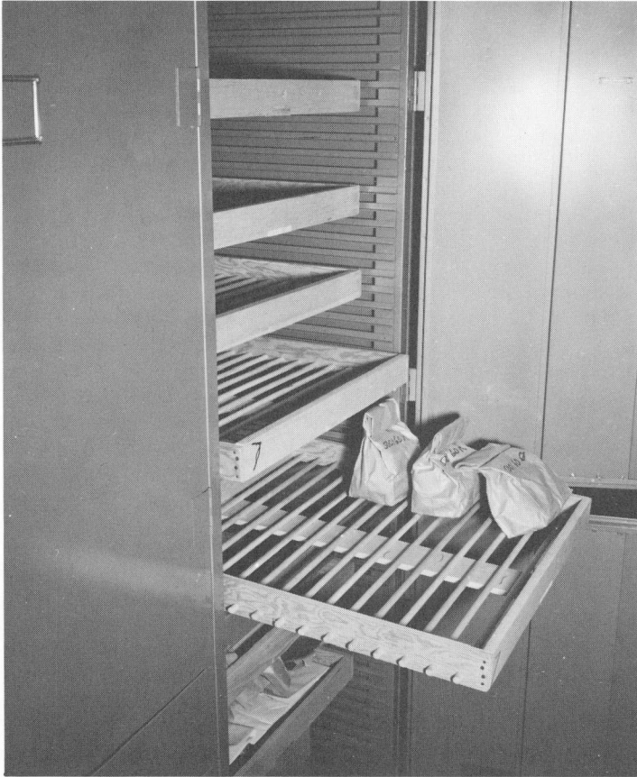
PLATE B 6. Interior of the Sample Preparation Trailer showing the drying racks within a drying cabinet.
