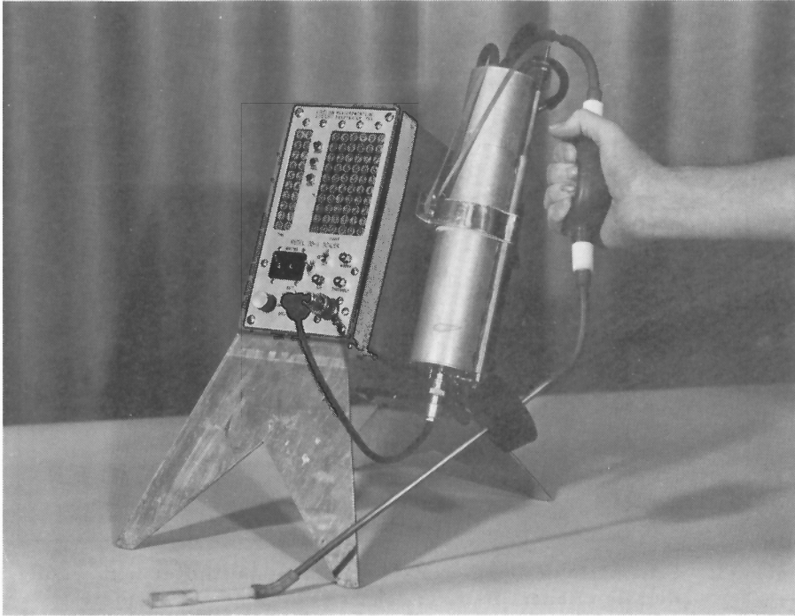
Figure 4. Photograph of radon detector equipped for on-site alpha activity measurements of soil gas emanations.
