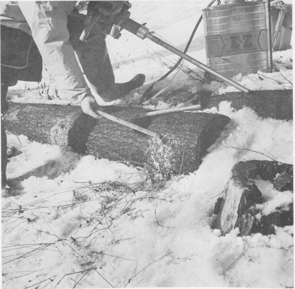
Figure 2. Taking 3/4-inch diameter cores with Geological Survey of Canada power-driven increment borer. (G.S.C. photo 201048-M)
