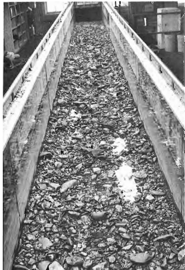
Figure 53.2. Upstream view of the flume working section. The bed shown is that formed in test 3. (GSC-203091-E)
