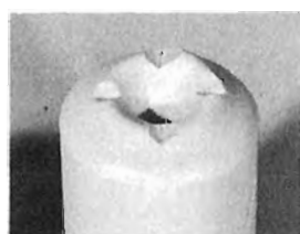
Figure 3. The vial, wax and the belemnite are ready for the pouring of the first half of the silicon rubber mould. But before pouring the rubber, an eyedropper or equivalent is positioned, 3 mm above the belemnite and a needle is pushed through it so as to guarantee its position above the belemnite. The eyedropper is removed during the pouring of the silicon rubber but it can easily be replaced after (Fig. 3b). The cavity created by the eyedropper will hold the reserve epoxy during centrifugation.
