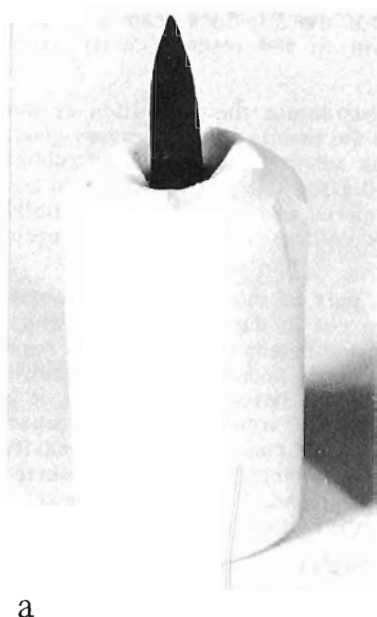
Figure 5. In Figure 5a the interface notches are carved with a razor-sharp knife after the silicon rubber and belemnite are removed from the plastic vial. Figures 5b and 5c show the two interface options discussed in the text.
