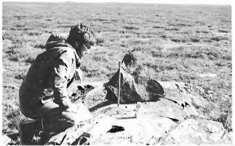
Figure 3. A typical benchmark installation on a bedrock outcrop, used to provide the control for accurate measurement of the vertical and horizontal movement of targets placed on mud boils. (GSC 203165-G)
