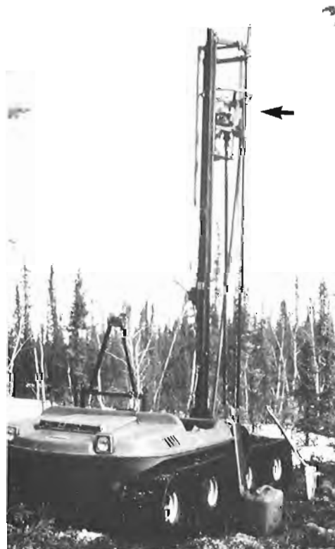
Figure 2. ATV-drill in drilling position; note the Stihl 4308 drill head (GSC 203314-F).
