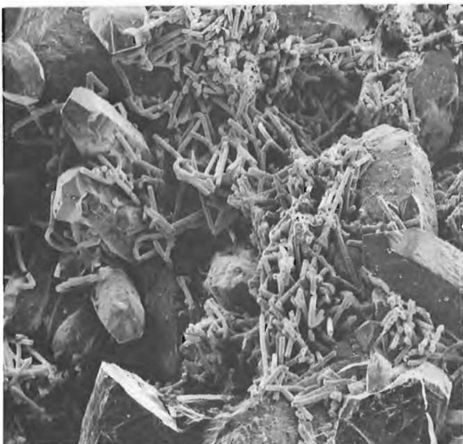
Figure 1. SEM photomicrograph of nests of duranusite on quartz. Field of view is 2.2 mm.
