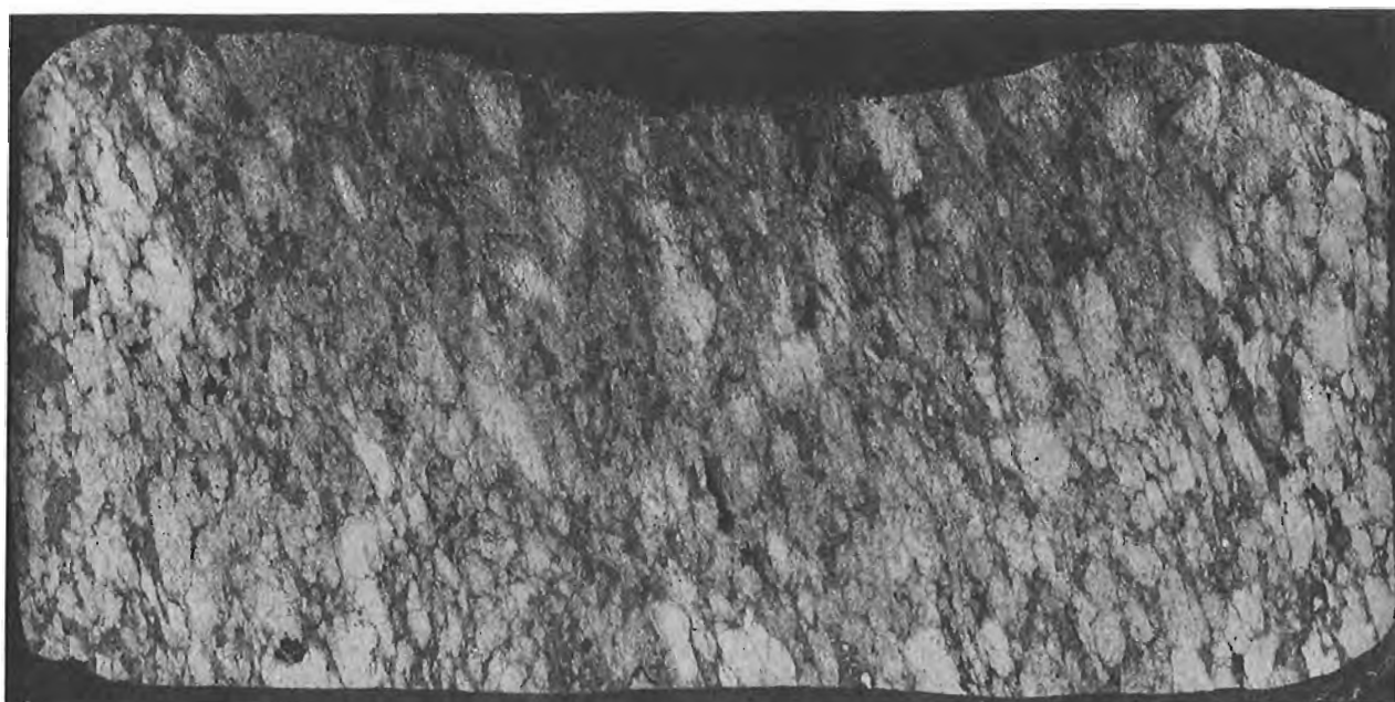
Figure 14.6c. Photomicrograph of quartzofeldspathic fragmental rock. Black interstitial material is sulphide. Sample 17-24, magnification is 4X, crossed nicols.
