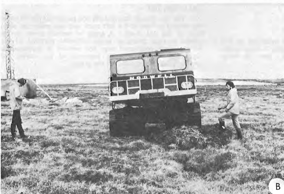
Figure 8.2 Test sites where normal stresses applied by a tracked vehicle were measured: A, site of the flat ground test. B, site of the hummocky terrain, side-on test. The site of the hummocky terrain, head-on test was similar to that of B. Note the channel formed by the track cleats which act as a guide for the bogie wheels.
